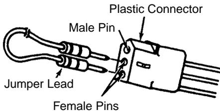
Method of jumping lead wires of connector plug from air flow switch.
